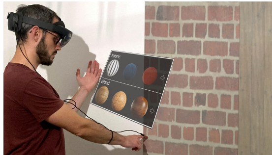
Fig. 6. Illustration of the texture augmentation in AR through an interior design scenario. A user wearing an AR headset and a wearable vibrotactile haptic device worn on their index is applying different virtual visuo-haptic textures to a real wall to compare them visually and by touch.
