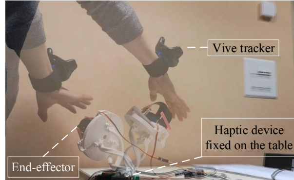
Figure 3.19 – Use case: encounter-type interaction with re-configurable surfaces. The motion of the user’s hand was tracked by the HTC Vive motion system. The base platform of the device was fixed on a table and the moving platform follows the hand so as to always face the user’s palm, ready for interaction.
