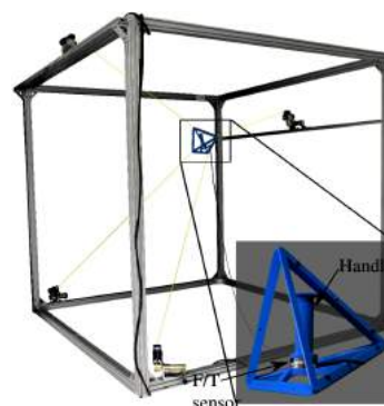
(h) haptic interface at Laval University [FCCG14]
