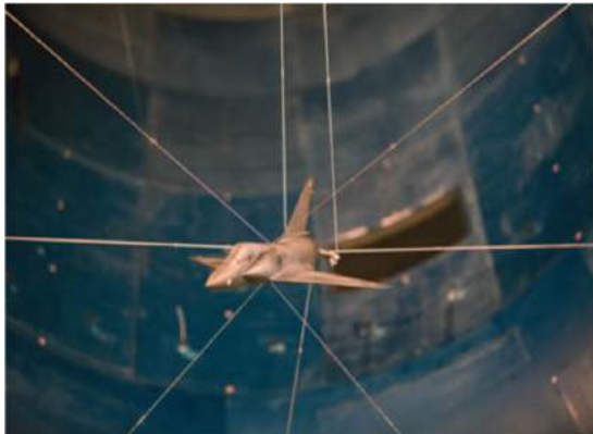
(c) A plane secured by a CDPR in a wind tunnel
