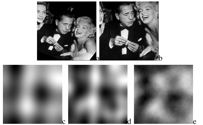
Figure 6. Simulated experiment: (a) initial image, (b) desired image, IDCT of the initial image for (c) K = 20 (d) K = 50 , (e) reconstructed image with the PCA with K = 50
