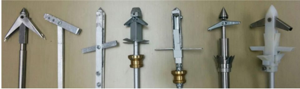
Figure 19. Harpoon tip and barbs design iteration.
