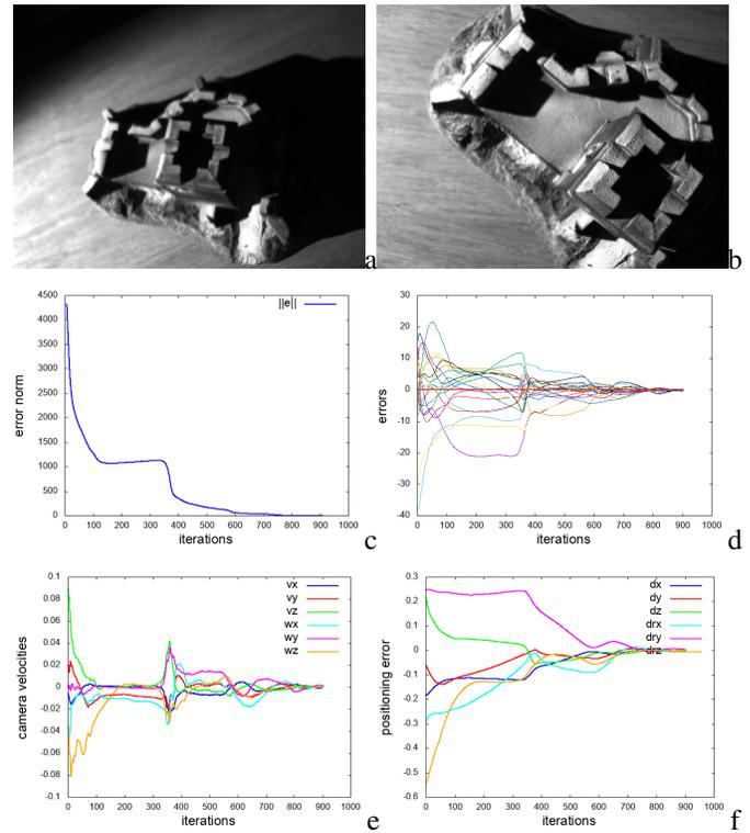
Figure 13. Experiment with a large 3D scene (a) initial image acquired by the camera  $\mathbf{I}(\mathbf{r})$ , (b) image  $\mathbf{I}^*$  acquired from the desired position, (c)  $\|\mathbf{w}(\mathbf{r}) - \mathbf{w}^*\|$  (d) errors  $\mathbf{w}(\mathbf{r}) - \mathbf{w}^*$  (e) camera velocity (in m/s and rad/s) (f) positioning error (in m and rad).
