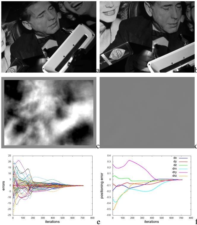
Figure 12. Experiment real scene with partial occlusions (a) initial image acquired by the camera  $\mathbf{I}(\mathbf{r})$ , (b) image  $\mathbf{I}^*$  acquired from the desired position, (c-d) error  $[\mathbf{U}\mathbf{w}(\mathbf{r})]_{50} - [\mathbf{U}\mathbf{w}^*]_{50}$  between reconstructed image for initial and desired position used for visualization but not used in the algorithm. (e) errors  $\mathbf{w}(\mathbf{r}) - \mathbf{w}^*$  (f) positioning error (in m and rad).
