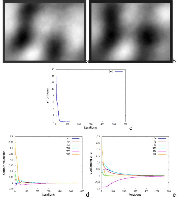
Figure 4. Experiment `exp-photo-rec`: Photometric visual servoing from the reconstructed image  $[\mathbf{U}\mathbf{w}(\mathbf{r})]_K$  with  $K = 20$ . (a) initial reconstructed image  $[\mathbf{U}\mathbf{w}(\mathbf{r})]_K$  (b) desired reconstructed image  $[\mathbf{U}\mathbf{w}^*]_K$  (c) error norm  $\|[\mathbf{U}\mathbf{w}(\mathbf{r})]_K - [\mathbf{U}\mathbf{w}^*]_K\|$  (d) camera velocity (in m/s and rad/s) (e) positioning error (in m and rad).
