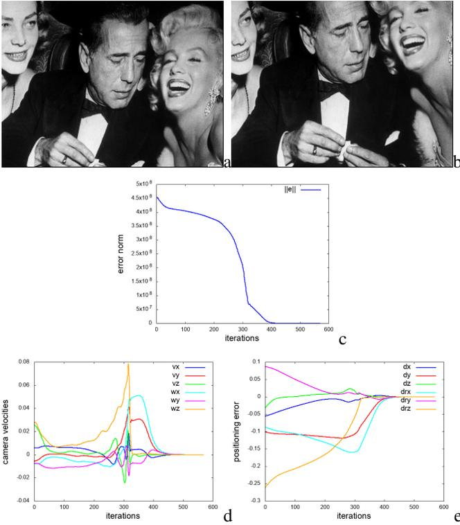
Figure 3. Experiment `exp-photo`: Photometric visual servoing [7]. (a) Initial image  $\mathbf{I}$  (b) desired image  $\mathbf{I}^*$  (c) error norm  $\|\mathbf{I}(\mathbf{r}) - \mathbf{I}^*\|$  (d) camera velocity (in m/s and rad/s) (e) positioning error (in m and rad).
