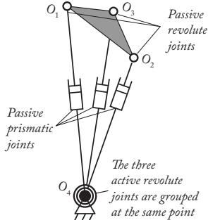
(a) in  $SE(2)$ , a 3-UPR planar parallel robot, i.e. a robot made of three identical legs made of an active revolute joint, followed by passive prismatic and revolute joints
