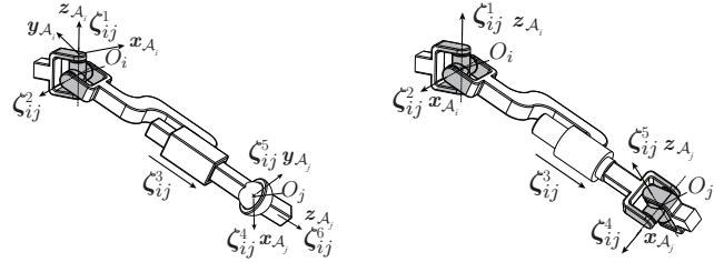
(a) Virtual kinematic chain corresponding to the case given in Fig. 1(a): a serial UPS chain
