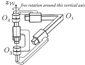
(a) Case 1: the equivalent mechanism has an internal mobility of two, i.e. an inflation plus a possible rotation around the line passing through  $O_2$  and  $O_3$
