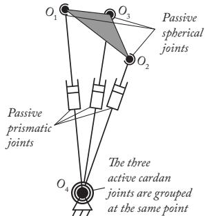
(b) in  $SE(3)$ , a 3-UPS spatial parallel robot, i.e. a robot made of three identical legs made of an cardan revolute joint, followed by passive prismatic and spherical joints
