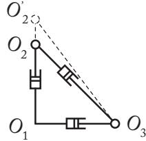
(b) Case 2: the equivalent mechanism has an internal mobility of two, i.e. an inflation plus a possible displacement of  $O_2$  (or  $O_3$ ) without moving  $O_3$  ( $O_2$ , respectively)
