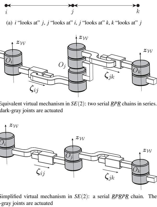
(b) Equivalent virtual mechanism in  $SE(2)$ : two serial RPR chains in series. The dark-gray joints are actuated
