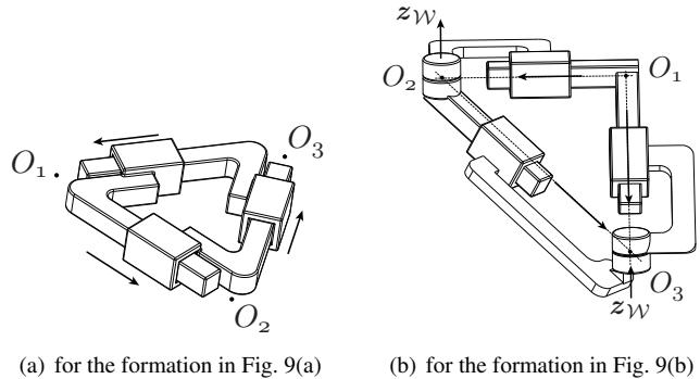
Fig. 10. Equivalent mechanical system.
