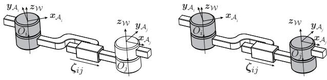
Fig. 2. Virtual (planar) kinematic chains corresponding to the elementary edges for  $SE(2)$ . The dark-gray joints are the actuated joints.
