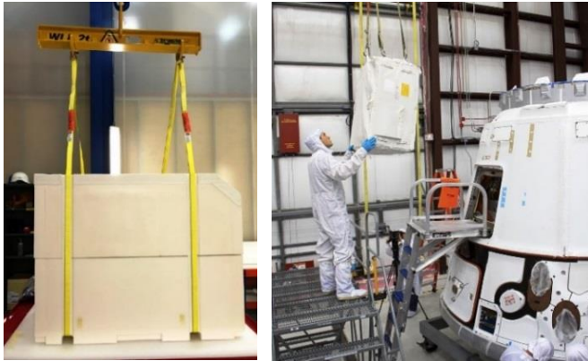
Figure 2 : Left: the clam shell (foam) that encompasses a RemoveDebris structural model, 2017. Right: loading of the Dragon capsule with a cargo bag. Credit: NASA, SpaceX from [44].
