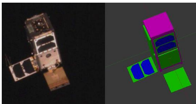
Figure 17: DSAT#1 Left: As seen by the camera, Right CAD model
