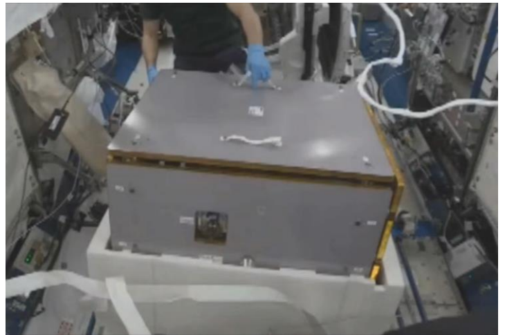
Figure 5: RmoveDEBRIS with its protective panels, is removed from the foam clamshell
