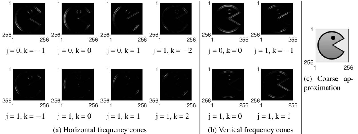
Figure 5: Non-subsampled shearlet decomposition at level 2 of the  $256 \times 256$  digital image shown in Fig. 2a. The parameter  $j$  denotes the scale of the corresponding shearlet filter while the shear parameter  $k$  controls its orientation. All coefficient matrices have the same size as the input image. The depicted decomposition is thus highly redundant with a redundancy factor of 13.
