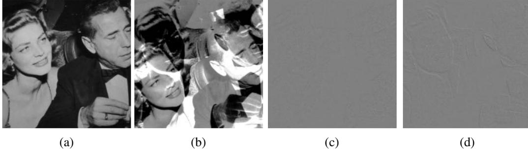
Figure 17: [scenario 1, test 2] (a) desired image  $\mathbf{I}^*$  (b) initial difference image  $\mathbf{I}_{diff}$ , (c) final difference image  $\mathbf{I}_{diff}$  in case of *s-wavelet* method, and (d) final difference image  $\mathbf{I}_{diff}$  in case of *s-shearlet* method.
