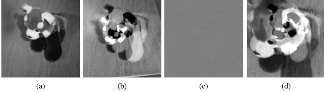
Figure 27: [*scenario 4, test4*] (a) desired image  $\mathbf{I}^*$  (b) initial difference image  $\mathbf{I}_{diff}$  (c) final difference image for *s-wavelet* method, and (d) that of *s-shearlet* method.
