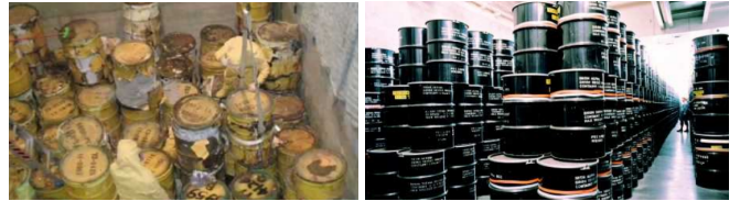
Fig. 1: Left figure: containers with unknown (or partially known) contents and mixed contamination levels that need to be examined, sorted and separated. Right figure: new special storage containers where contaminated waste must be placed.
