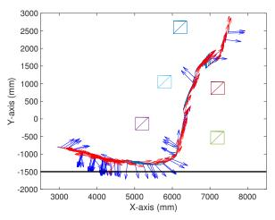
Fig. 2: Layout of the assessment course showing obstacles (rectangular cardboard boxes), the wheelchair's travel direction (red arrow) and the user's command direction (blue arrow) when driving with PSC. The thick black line represents a wall. Qualitatively, PSC is able to compensate for erroneous user input and generate a safe, smooth trajectory.
