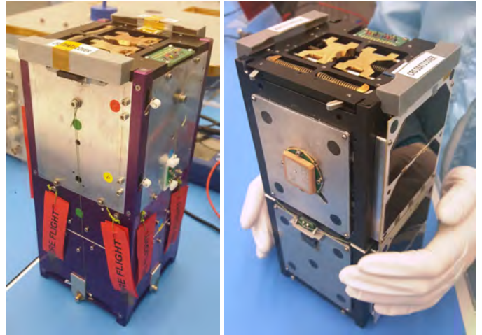
Fig. 7: CRS insertion on to CubeSats. This figure shows DS-1 (left) and DS-2 (right) with the CubeSat Release Systems (CRS) attached (on top).
