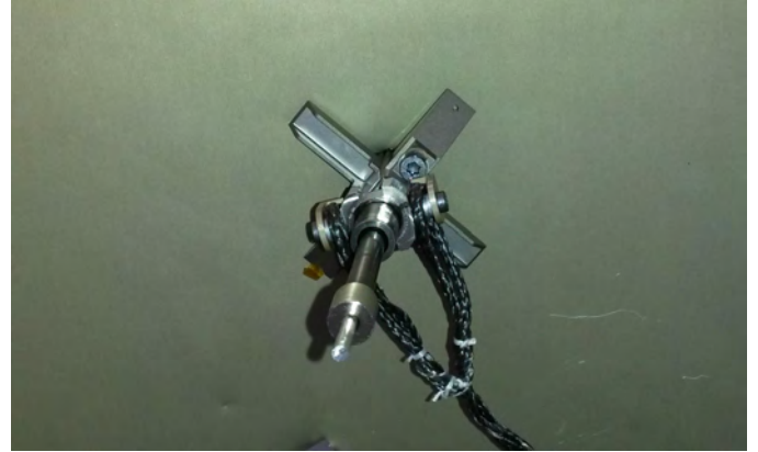
Fig. 15: Harpoon Impact . This figure shows a harpoon impacted into a target.
