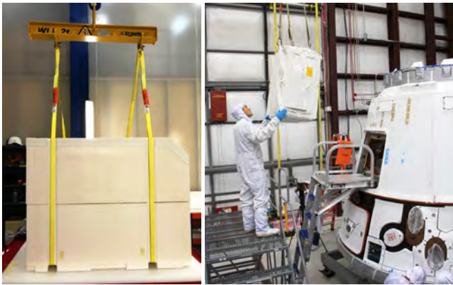
Fig. 22: Clam Shell. Left: the clam shell (foam) that encompasses a RemoveDebris structural model. Credit: SSTL, 2017. Right: loading of the Dragon capsule with a cargo bag. Credit: NASA, SpaceX from [42].
