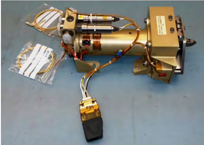
Fig. 18: FM Harpoon Payload. Showing the harpoon payload (no MLI) without the harpoon target or casing.
