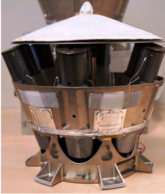
Fig. 10: FM Net . This figure shows the final net flight model with ejection springs unloaded.
