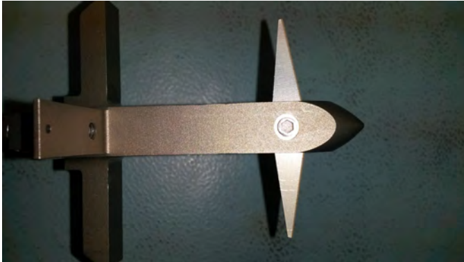
Fig. 14: Harpoon Barb Mechanism . This figure shows the projectile with the barbs deployed.
