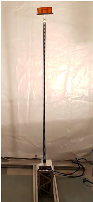
Fig. 17: FM Boom - Deployed. This figure shows the harpoon target assembly (HTA) and the boom fully deployed to 1.5 m with gravity assistance.
