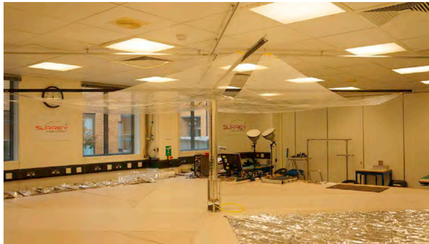
Fig. 33. Dragsail: Deployment Test. With EQM unit.
