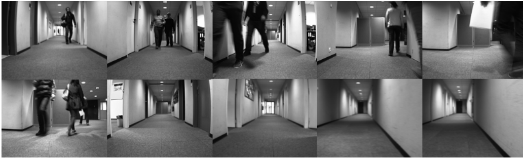
Figure 6.13 – Changes in the navigation environment from the mapped one: people passing by, opening of the doors, change in the local illumination due to a dead bulb and blur in the image.
