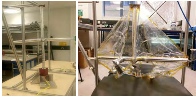
Fig. 11: DS-1: Inflatable Functional Testing. Left: inflation testing from SQM without sail segments. Right: inflation testing from SQM with sail segments attached (mid-inflation). Both tests using external gas supply line.
