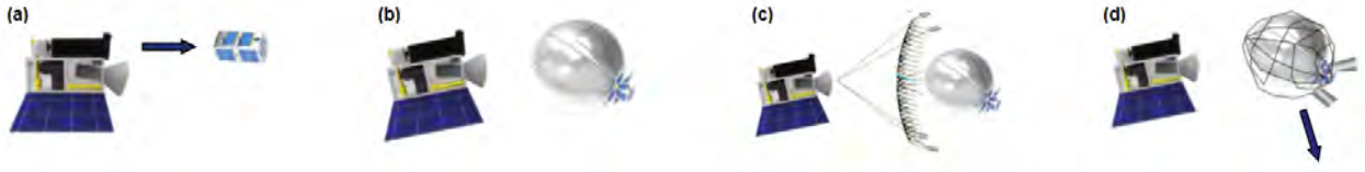
Fig. 1: Net Experiment. This figure shows the sequence in the net experiment: (a) DS-1 CubeSat ejection, (b) balloon inflation, (c) net capture, (d) deorbiting.
