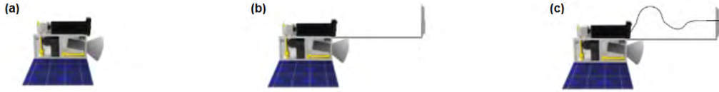
Fig. 2: Harpoon Experiment. This figure shows the sequence in the harpoon experiment: (a) initial configuration, (b) deployable target deployed, (c) harpoon capture.
