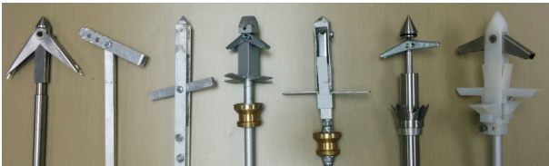
Fig. 24: RemoveDebris Projectile Prototypes and Evolution.
