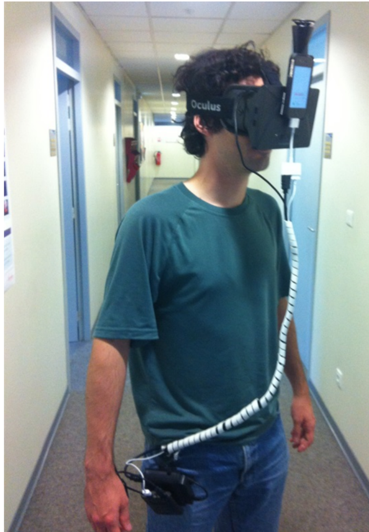
Figure 2.7 – FlyVIZ V2. The second iteration of the prototype uses a smartphone, a compact catadioptric lens and an Oculus Rift HMD.
