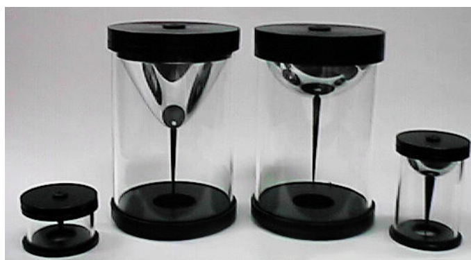
Figure 1.15 – Various mirrors suitable to build catadioptric sensors. The picture does not show the additional lens needed to build a functional optical system.
