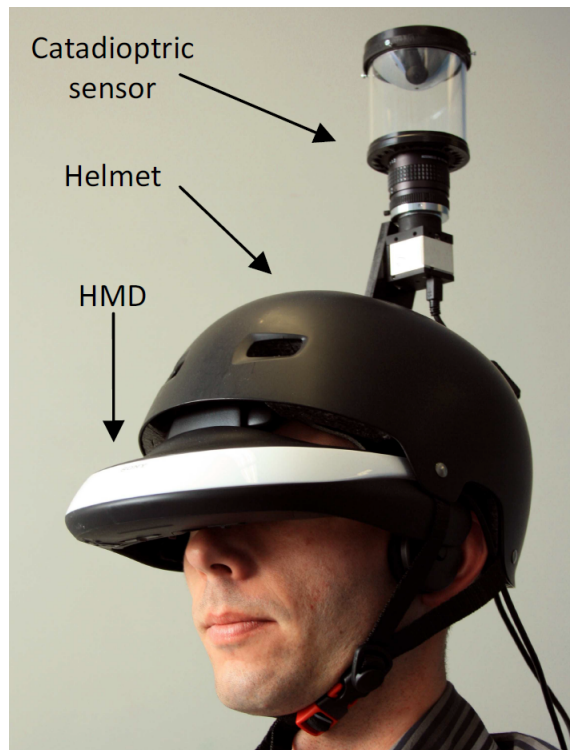
Figure 2.1 – FlyVIZ prototype and proof-of-concept.
