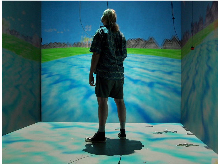
Figure 1.21 – The CAVE (Cave Automatic Virtual Environment). The user is surrounded by planar screens where images are projected. The views are computed dynamically with respect to perspective projections computed taking the position of the user's eyes into account [CruzNeira 93].
