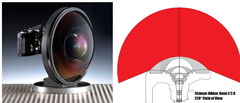
Figure 1.13 – Fisheye lens. The model shown is a Nikon 6mm fisheye lens. It weighs 5.2kg and captures field-of-view of 220^\circ . The schematic on the left shows the lens arrangement used to collect light ray coming from behind the lens
