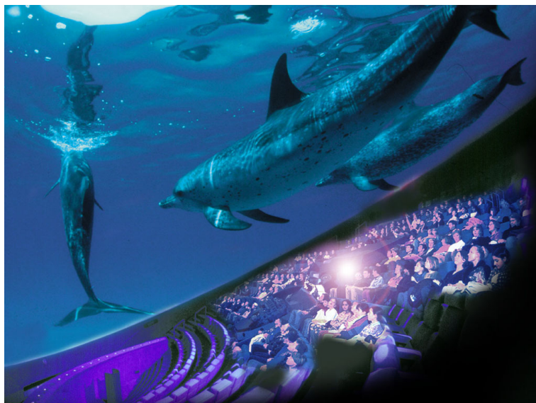
Figure 1.22 – An IMAX Dome theater. Images are projected on a hemispherical screen with a fish-eye lens.
