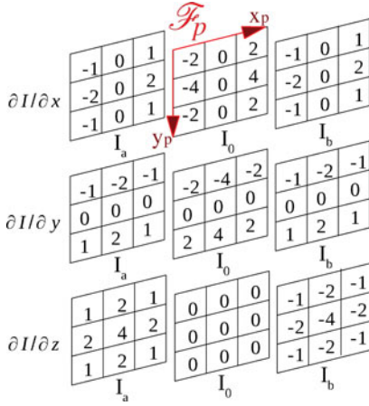
Fig. 3. Three filters are applied on each pixel of the current image I_0 to compute the gradient components ( \nabla I_x, \nabla I_y, \nabla I_z ) using the additional parallel images I_a and I_b acquired on both sides of I_0 .
