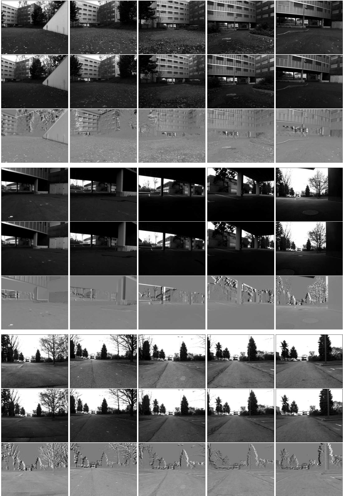
Figure 12: Outdoor navigation experiment, beginning of the experiment. First row: current image acquired by the vehicle, second row: desired image and third row: difference between the current and desired image. The first top column and the last bottom column show respectively the first images and the last images used in the navigation task.
