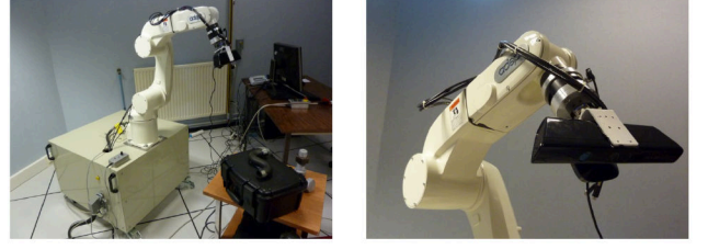
Fig. 3. ADEPT Viper robotic system equipped with a Microsoft Kinect sensor.
