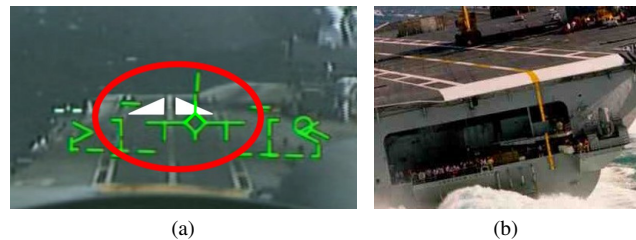
Fig. 1. (a) Pilots try to put the HUD velocity vector at the basis of the triangle mark in order to follow the glide slope; (b) The angle between the drop and the alignment lines (yellow and dash) provides lateral information
