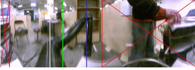
Fig. 4. Panoramic view provided to the user before the arm positioning. Red crosses: positions that can not reach the first joint. White line: first axis position. Blue line: initial FOV of the camera (left picture of Fig 3). Green line: desired camera direction, given by the user with one click. After the arm positioning, the embedded camera gives the right picture of Fig 3.
