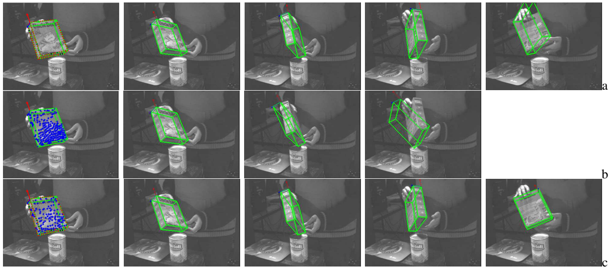
Fig. 4. Rice box sequence. Images for (a): the edge-based tracker, (b): the texture-based one, (c): the hybrid one. Only the hybrid tracker succeeds to track correctly the object all along the sequence, despite the specularities and the misleading environment. The grey level samples are represented in the first image by blue crosses and the edge location by red points.
