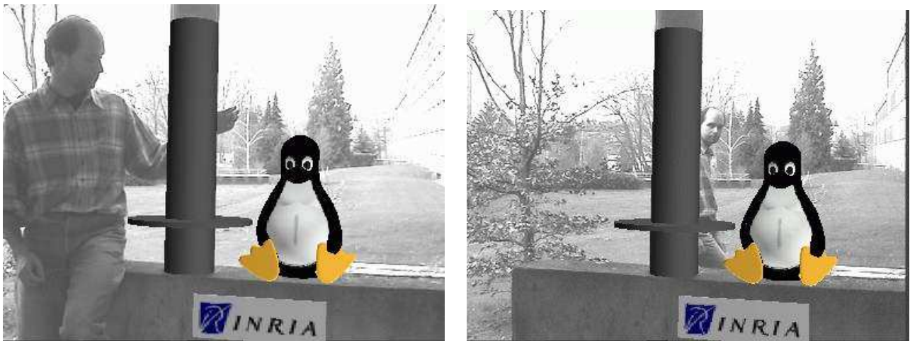
Figure 6.21: Tracking considering a cylinder and two straight lines with application to augmented reality.
