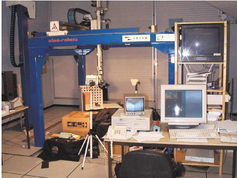
Fig. 11. Experimental setup at IRISA/INRIA Rennes: six degrees of freedom cartesian robot with a camera mounted on the end-effector.
