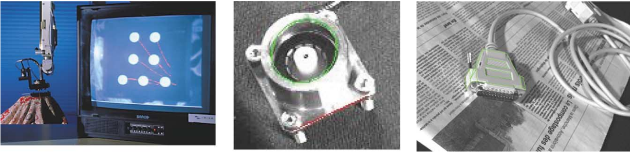
Fig. 1. Tracking features for visual servoing robotic tasks — three levels of complexity: (a) tracking artificial landmarks (white dots) for a grasping task; (b) tracking specific geometrical features (ellipse and segment); (c) tracking complex objects (a connector) in a textured environment.
