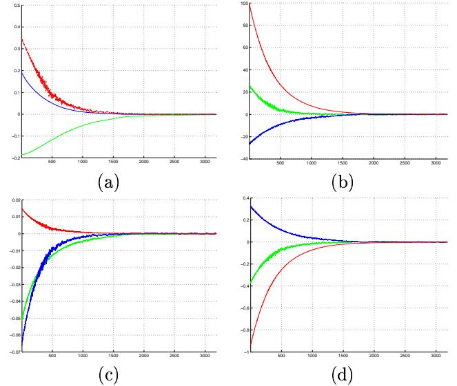
Figure 6: Error on extended image coordinates (a),  $u\theta$  (dg) (b), translational velocity  $\mathbf{V}$  (cm/s) (c) and rotational velocity  $\Omega$  (dg/s) (d) versus iteration number
