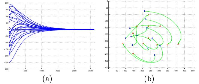
Figure 5: Error on pixels coordinates (a) and trajectory (b) of the target points
