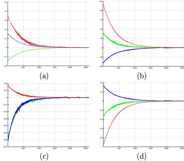
Figure 4: Error on extended image coordinates (a),  $u\theta$  (dg) (b), translational velocity  $\mathbf{V}$  (cm/s) (c) and rotational velocity  $\Omega$  (dg/s) (d) versus iteration number
