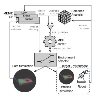
Fig. 1. System's architecture. The action database contains MENID rules updated with experiences from both the simulated and the target environments. In turn, the execution history of the action is used for optimal decision making. The environment selection criteria for a given action depends on: (1) the simulator's accuracy; and (2) the confidence in the action's empirical outcome distribution.
