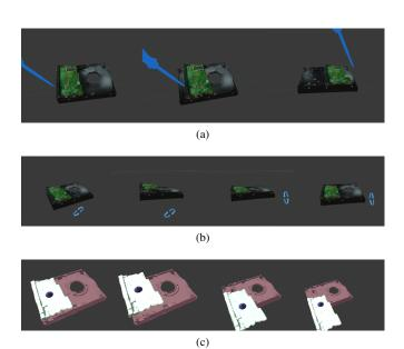
Fig. 3. Illustration of the three scenarios: (a) First scenario: the lever (blue) is used to remove the PCB (green) from the bay; (b) Second scenario: different shaking angles are applied to the bay to remove the PCB from it; (3) Third scenario: the PCB (white) is removed from the bay (red) using a suction cup (in black, located on the PCB).
