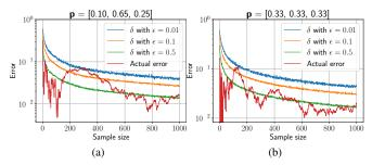
Fig. 2. Error bounds ( $\delta$ ) for the estimation of two categorical distributions as sample size increases. The actual error is calculated as  $\max_i |j_{p_{r,i}} - j_{q_{r,i}}|$ . Notice that, in both (a) and (b), the bounds follows quite closely the trend of the error. Moreover, the bounds with  $\varepsilon = 0.01$  and  $\varepsilon = 0.1$  are seldom exceeded. The worst case scenario analyzed by Thompson (uniform distribution) is shown in (b).
