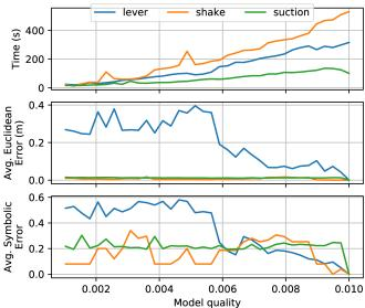
Fig. 4. Different performance measures for the *lever*, *shake* and *suck* action as the quality of the models (i.e. proportion of retained vertices) varies.
