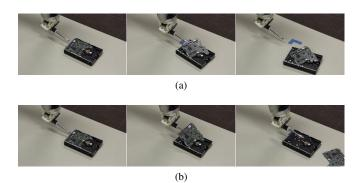
Fig. 5. Two different lever motions for levering and removing a PCB from the hard drive reproduced with the robot arm. The first motion, (a), is unsuccessful, while the second, (b), is successful.
