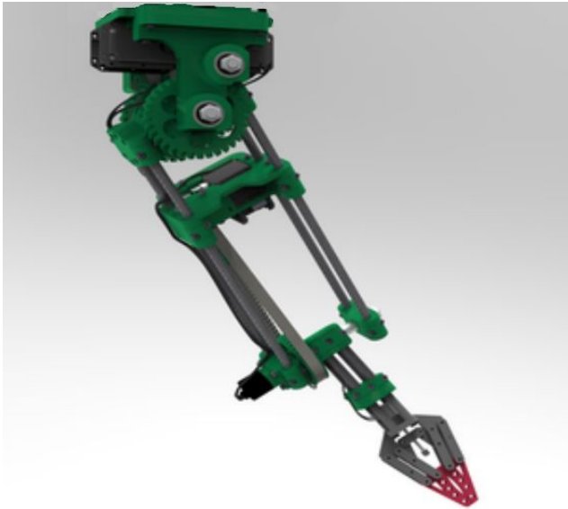
Mechanical design of the 3-DoF arm realised at LAAS.
