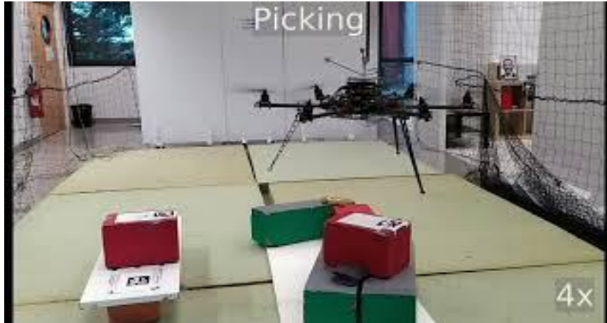
Experiments at LAAS: Autonomous pick-and-place application. G. Corsini et al.. A General Control Architecture for Visual Servoing and Physical Interaction Tasks for Fully-actuated Aerial Vehicles. AIRPHARO 2021.
