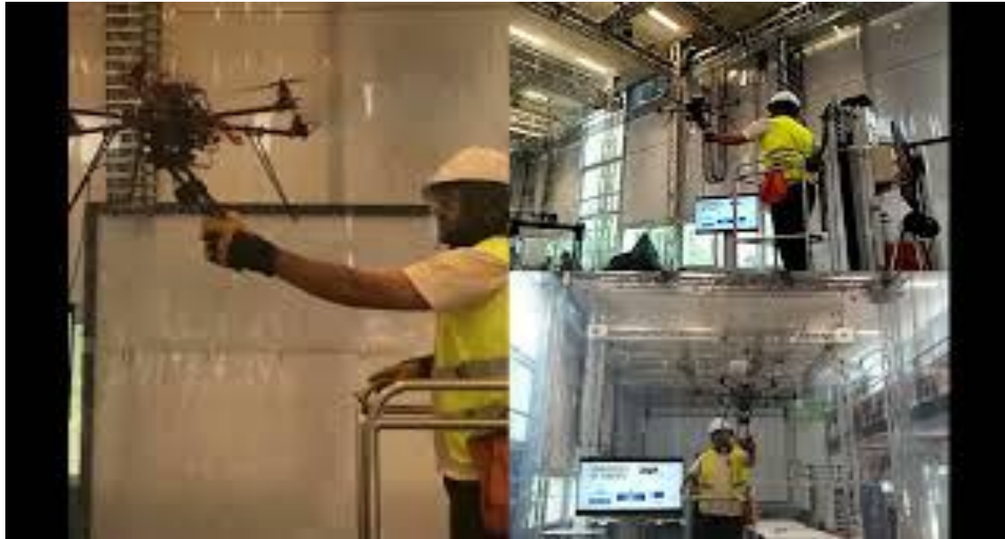
Experiments at University of Twente (the Netherlands): human-to-aerial-robot handover. A. Affi et al., Physical Human-Aerial Robot Interaction and Collaboration: Exploratory Research, IEEE International Conference on Human-Machine Systems (ICHMS) , 2022.
